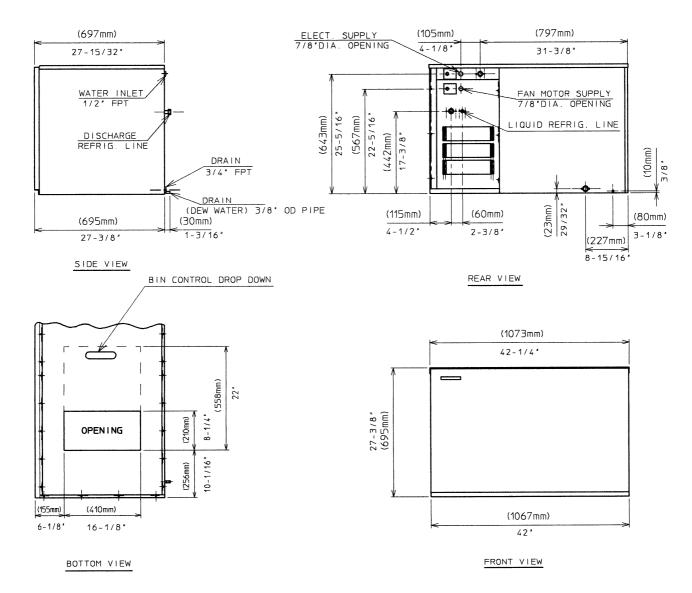
Note: When used with a storage bin not recommended by Hoshizaki, the icemaker needs the space at the bottom opening as in the illustration.
